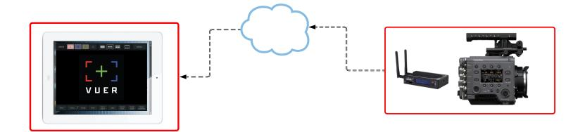
This allows a mobile device to connect to an 'Access Point 'network created by the Teradek Cube. The benefit of using an 'Access Point' network is you do not have to keep connecting multiple devices to local wifi networks if your shoot is moving locations. Set up and maintenance is argueably much easier.
